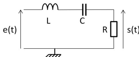
$$\underline{H} = \frac{jRC\omega}{1 + jRC\omega - LC\omega^2} \quad \text{avec} \quad H_0 = 1 \quad \omega_0 = \frac{1}{\sqrt{LC}} \quad \sigma = \frac{R}{2} \sqrt{\frac{C}{L}} \quad Q = \frac{1}{R} \sqrt{\frac{L}{C}}$$
