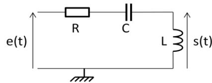
$$\underline{H} = \frac{-LC\omega^2}{1 + jRC\omega - LC\omega^2} \quad \text{avec} \quad H_0 = 1 \quad \omega_0 = \frac{1}{\sqrt{LC}} \quad \sigma = \frac{R}{2} \sqrt{\frac{C}{L}}$$
