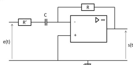
$$v_- - e(t) = -(R' + \frac{1}{jC\omega})i(t) \quad v_+ = 0 \quad s(t) - v_- = -Ri(t) \Rightarrow \underline{H} = -\frac{jRC\omega}{1 + jR'C\omega}$$
