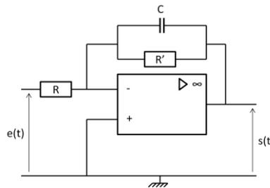
$$v_- - e(t) = -Ri(t) \quad v_+ = 0 \quad s(t) - v_- = -\left( \frac{1}{\frac{1}{R'} + jC\omega} \right) i(t) \Rightarrow \underline{H} = -\frac{R'}{R} \left( \frac{1}{1 + jR'C\omega} \right)$$
