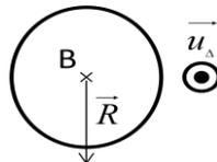
$$M_{\Delta} = \vec{M}_A \cdot \vec{u}_{\Delta} = (\vec{R} \wedge \vec{BA}) \cdot \vec{u}_{\Delta} = (\vec{R} \wedge (\vec{BH} + \vec{HA})) \cdot \vec{u}_{\Delta} = (\vec{R} \wedge \vec{BH}) \cdot \vec{u}_{\Delta} \Rightarrow |M_{\Delta}| = \|\vec{R}\| \cdot BH$$
