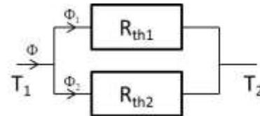
$$R_{th1\parallel 2} = \frac{R_{th1}R_{th2}}{R_{th1} + R_{th2}}$$
